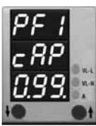
If the displacement is NEGATIVE (capacitive) the indications on the display will be <cap> and a point on the right lower side will be lights-on.
