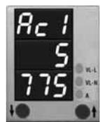
Measurement of Active Power in Watt.
