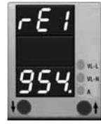
If on the right side of the value, a little point lights-on it means that the value is NEGATIVE, so the measured value is CAPACITIVE instead of INDUCTIVE.
