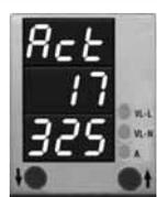
Measurement of Active Power in Watt.
