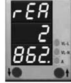
If on the right side of the value, a little point lights-on it means that the value is NEGATIVE, so the measured value is CAPACITIVE instead of INDUCTIVE.
